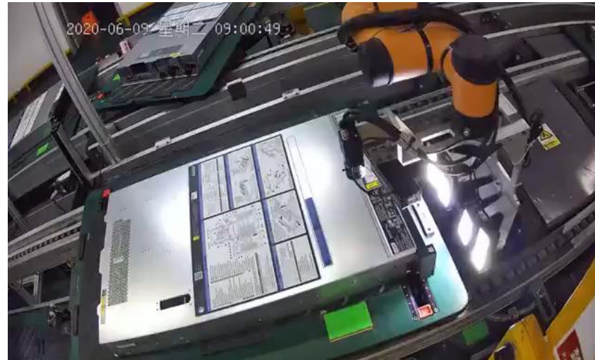
Server Appearance Detection(Lenovo)
